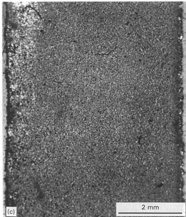
Figure 7 Low-magnification microstructural comparisons of SHS TiC preforms (Micron Ti-020/Alfa 00641) illustrating the effect of sample outgassing and colloidal processing methods on improving product uniformity: (a) ultrasonically-mixed and uniaxially-cold pressed, 34.5 MPa, not outgassed; (b) same as (a) but samples were outgassed; (c) pressure-cast and outgassed.
